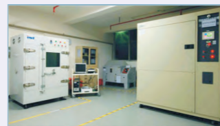
Faster temperature chamber & Thermal Shock Test Chamber
